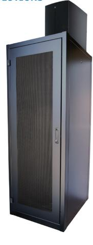
R. F. Mote Chimney Ducted cabinets are typically configured with perforated front door and solid rear door. Top duct work directs hot exhaust air either to the rooms drop ceiling, which acts like a hot plenum, or directly to HVAC ductwork that further directs the airflow to the intakes of the CRAC/CRAH units.
